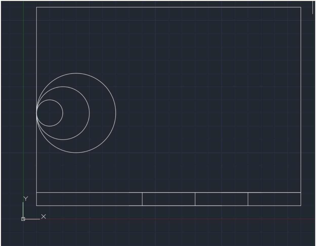
5. Draw a fourth circle using the CIRCLE command in the command line with the center at  $(2.5, 4.5)$  and the radius is 2 inches.
