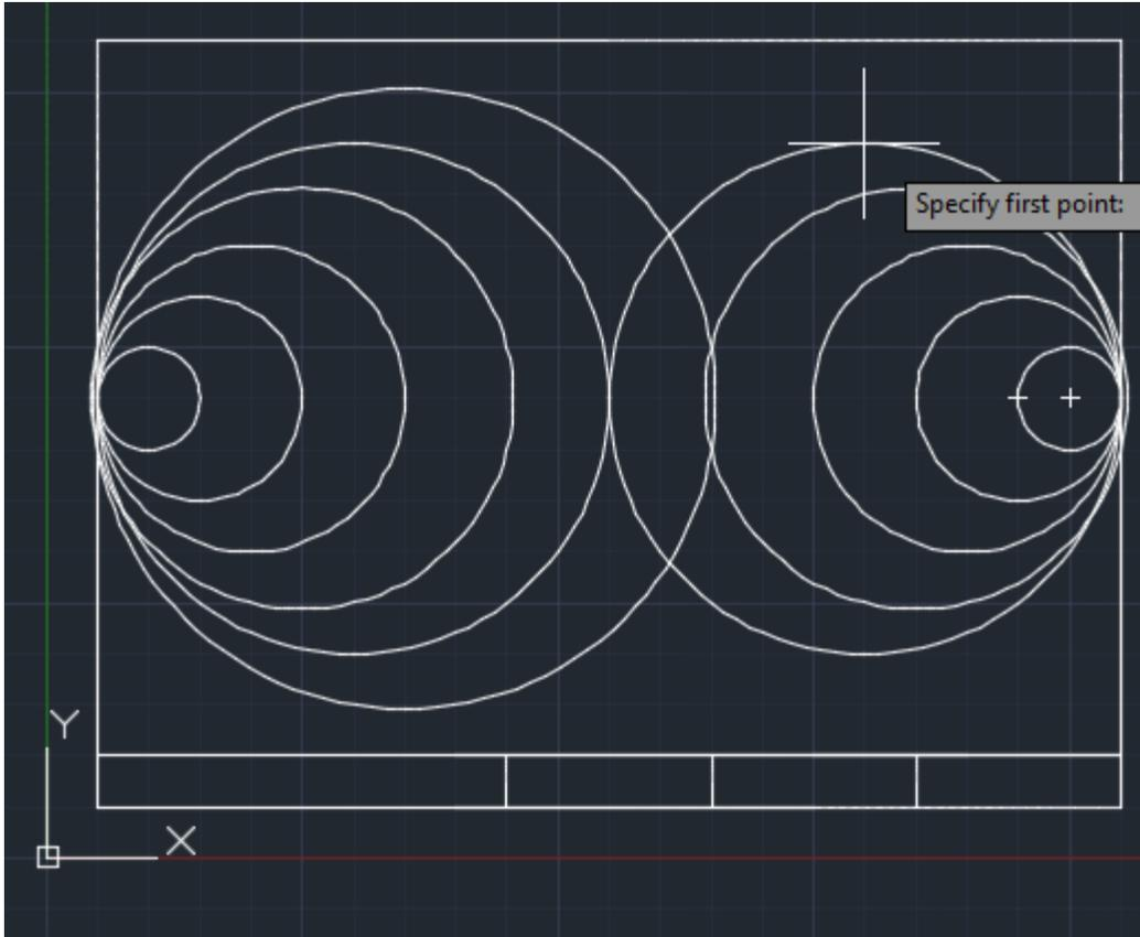
13. Create a circle by typing CIRCLE into the command line with a center of (7.5, 4.5) and a radius of 3 inches
