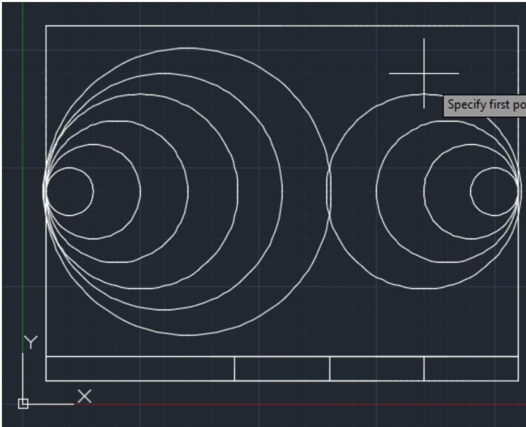
12. Create a circle by typing CIRCLE into the command line with a center of (8, 4.5) and a radius of 2.5 inches.
