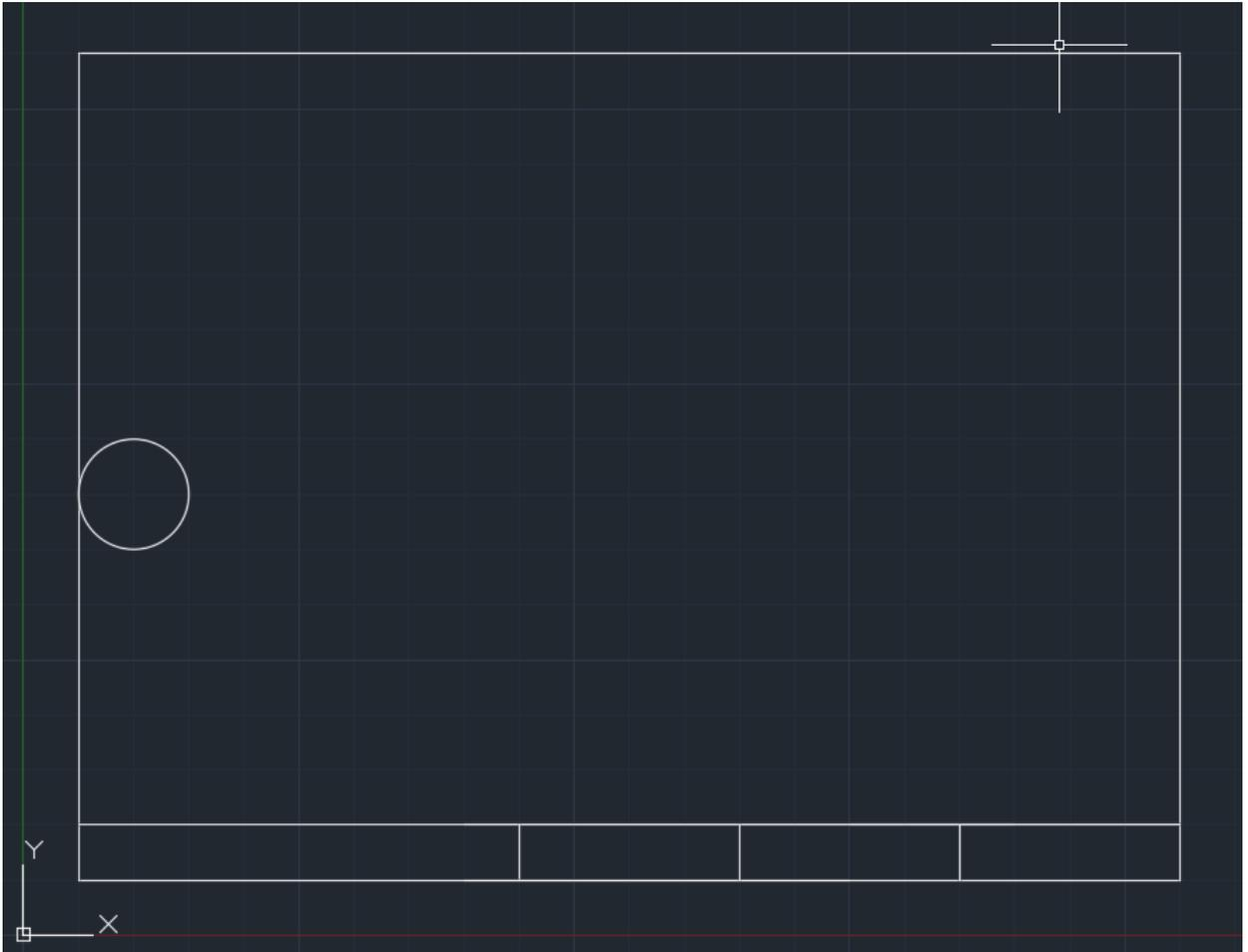
3. Draw a second circle using the CIRCLE command in the command line, the center is at the point (1.5, 4.5) and the radius being 1 inch.
