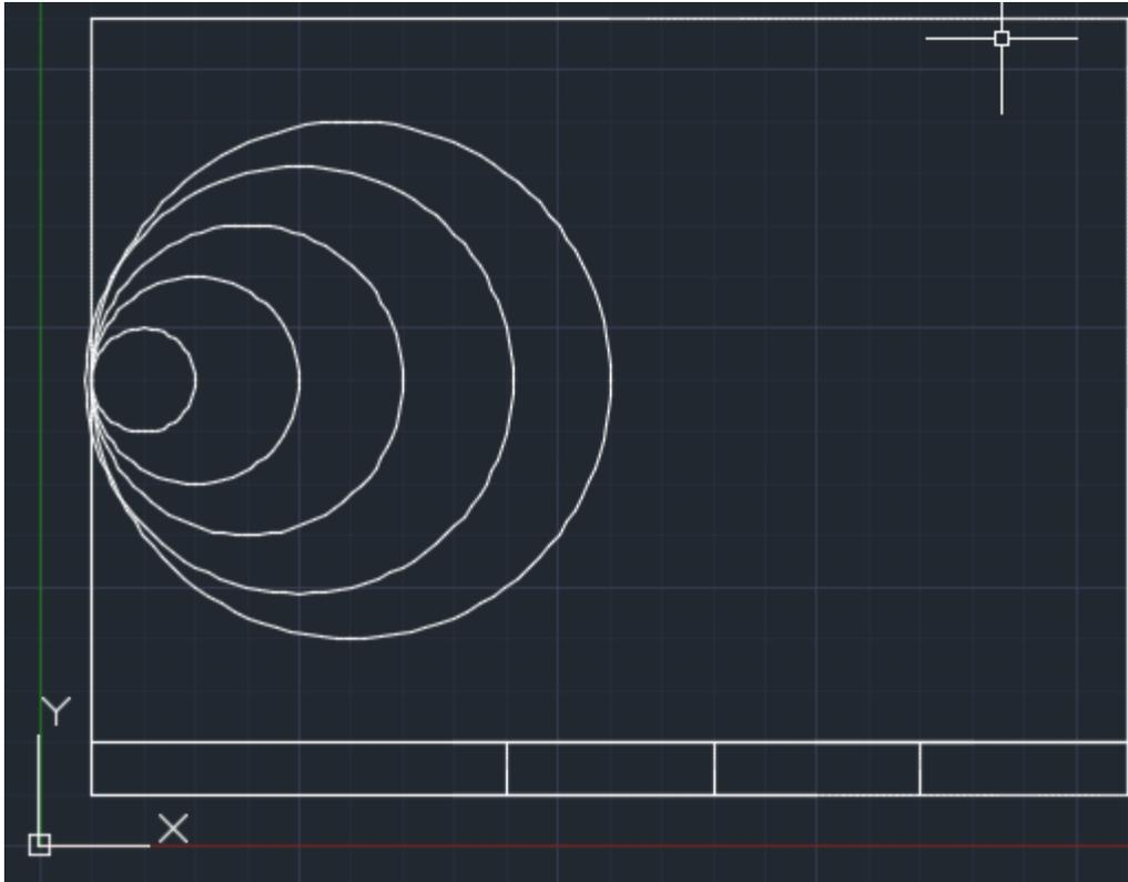
7. Draw a sixth circle using the CIRCLE command in the command line with a center of (3.5, 4.5) and a radius of 3 inches.
