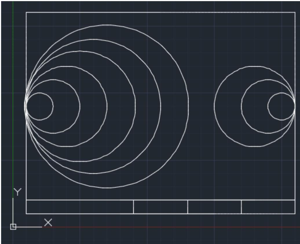
11. Create a circle using the command line with a center by typing in CIRCLE into the command line with a center of (8.5, 4.5) and a radius of 2.
