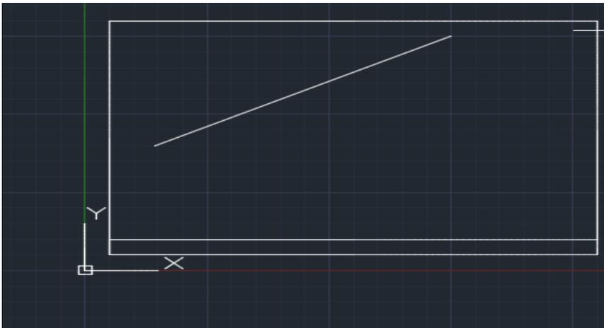
3. Begin the line tool again in the command bar `LINE` select previous for the starting point, along with 7 for the length and (hold tab) an angle of 15.
