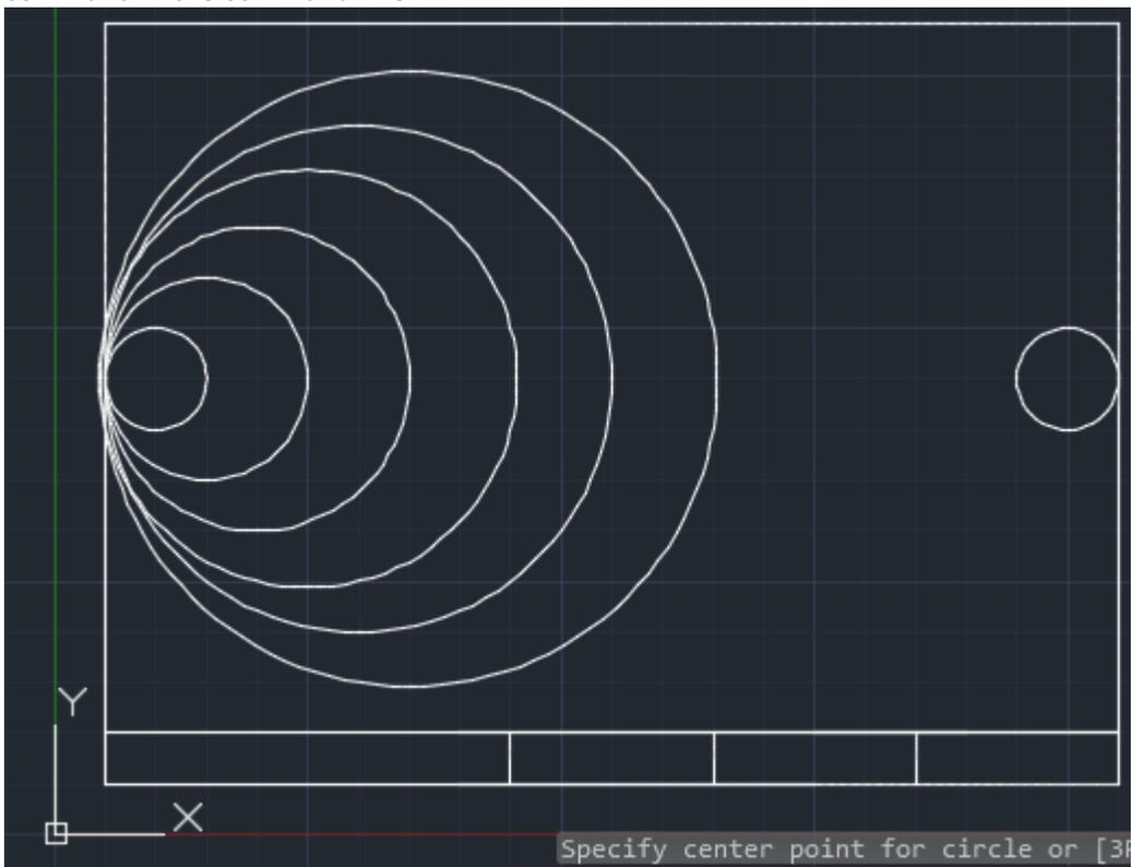
9. Create a circle using the command tool with the center (9.5, 4.5) with a radius of 1 using the CIRCLE command in the command line.
