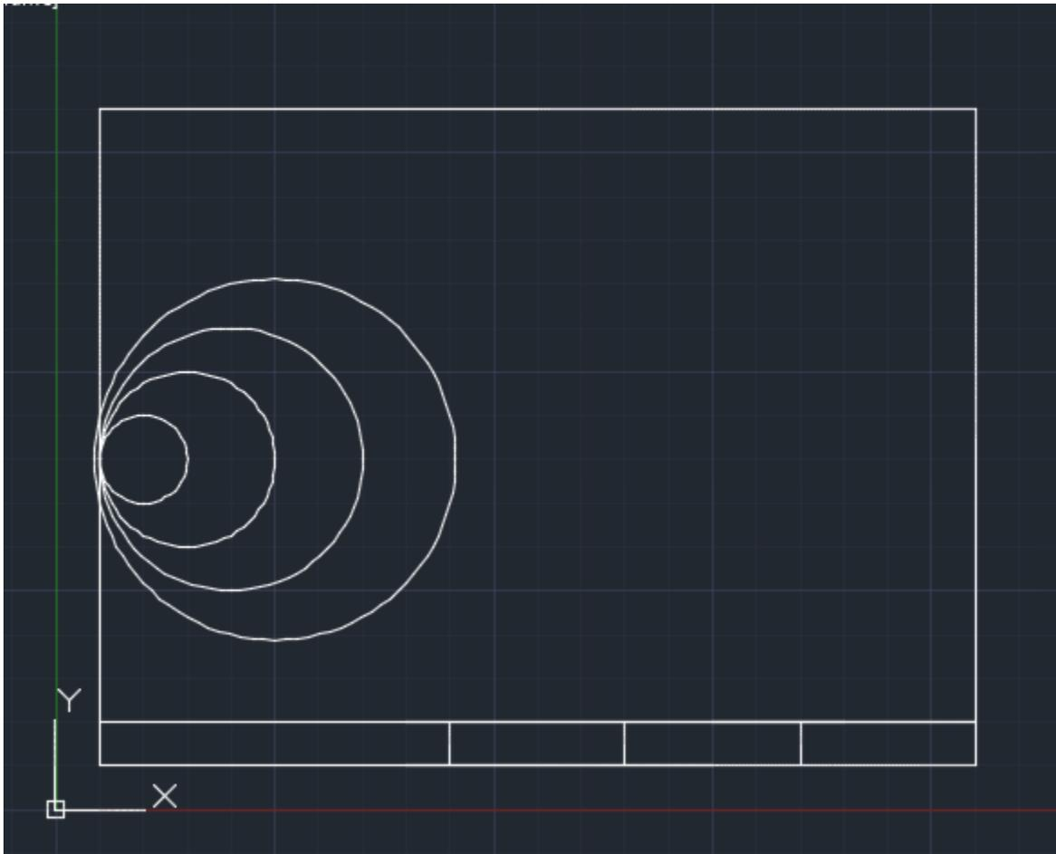
6. Draw a fifth circle using CIRCLE command in the command line with a center at (3, 4.5) and the radius being 2.5 inches.
