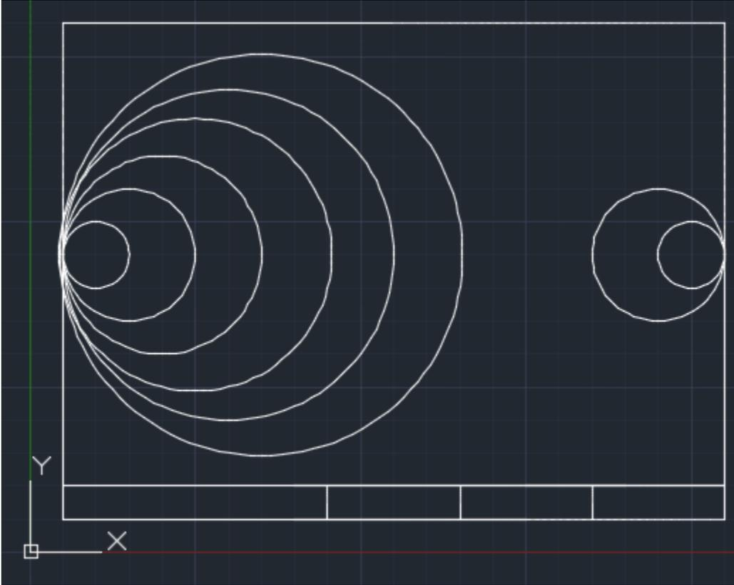
10. Create a circle using the command tool with the center (9, 4.5) with a radius of 1.5 using the CIRCLE command in the command line.
